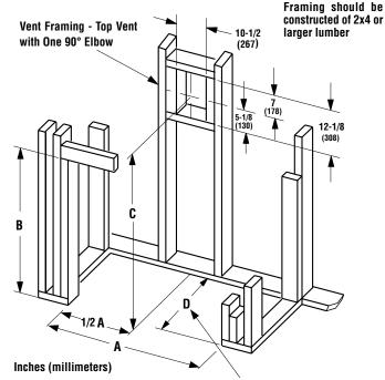
Dimension "D" is the required framing depth when the finish material (drywall) thickness is 1/2 in. (13mm).
